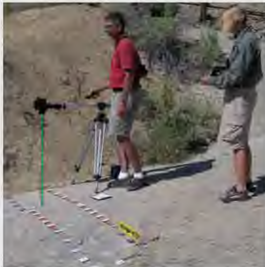
Figure A.5. It is important for the camera to maintain a consistent relation to the subject. Keeping a perpendicular angle to the subject is preferable. The dashed line represents the ray described in Appendix Figure A.4. A tripod with an extension arm was used when photographing a dinosaur trackway at the Red Gulch Dinosaur Tracksite, Wyoming.
